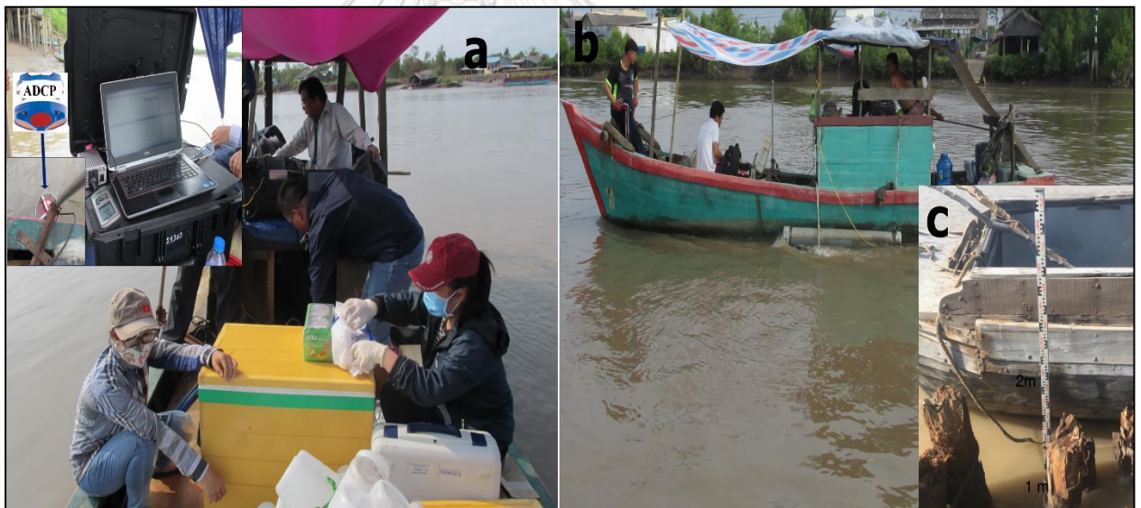
Figure 0.6 Data collection on the field: (a) water sample collection, velocity and bathymetric measurements, (b) water discharge measurement at the upstream, and (c) water level measurement at downstream of the river.
