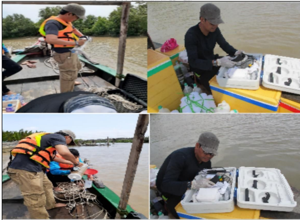
Figure 0.4 Surface water collection and in-situ measurement on the field
