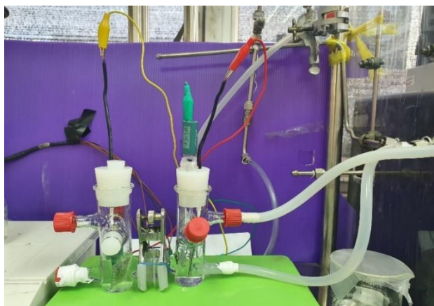
Figure 29 Schematic of CO 2 RR setup at Chemical Engineering, Chulalongkorn University.
