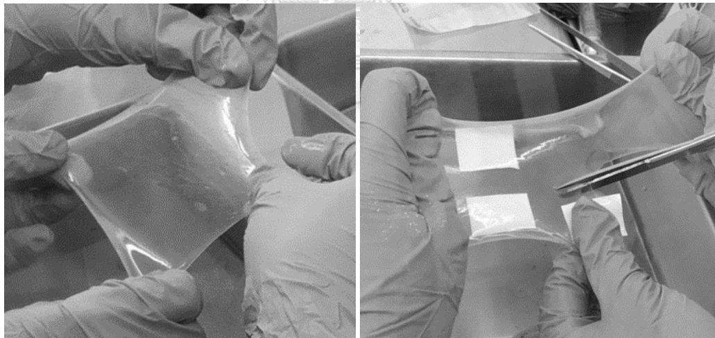
Figure 6: Photograph of CAM (A) after washing and (B) cutting to size with nitrocellulose membranes attached.
