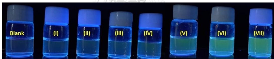
Figure 3.23 Fluorescence images of EC@Naph nanosensors (3.5% v/v) obtained by adding different concentrations of nonanal (in DMSO): blank ( EC@Naph ), (I) 1 \mu\text{M} , (II) 5 \mu\text{M} , (III) 10 \mu\text{M} , (IV) 50 \mu\text{M} , (V) 100 \mu\text{M} , (VI) 1.0 mM, and (VII) 1.5 mM.
