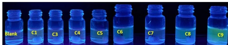
Figure 3.21 Fluorescence images of EC@Naph nanosensors with the addition of different aldehyde species (2 mM in DMSO) including the blank ( EC@Naph ), (C1) formaldehyde, (C3) propanal, (C4) butanal, (C5) pentanal, (C6) hexanal, (C7) heptanal, (C8) octanal, and (C9) nonanal. The measurements were conducted in 20 mM acetate buffer at pH 5.0 under a 365 nm UV irradiation 42 .
