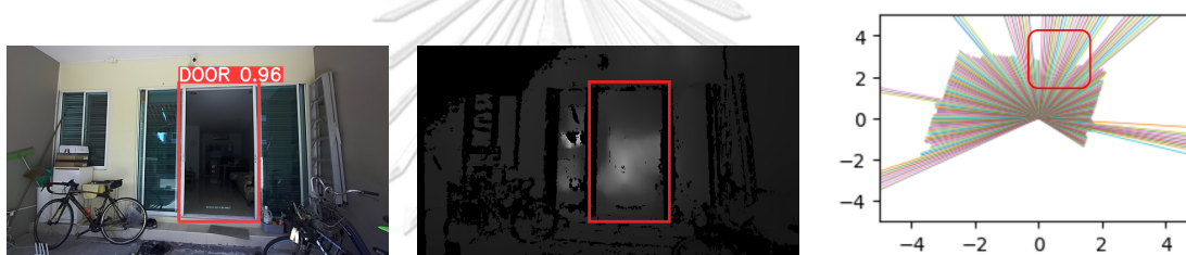
Figure 4.3: Image on the left shows a door detection on a rectified RGB image. The image in the middle shows the associated detected door on the depth registered image. The image on the right shows the associate door (labeled as a red square) in the laser scan.
