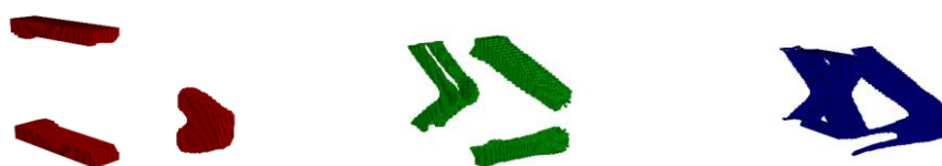
(a) 3D cantilever design based on three volume constraints at final stage (105 iterations).
