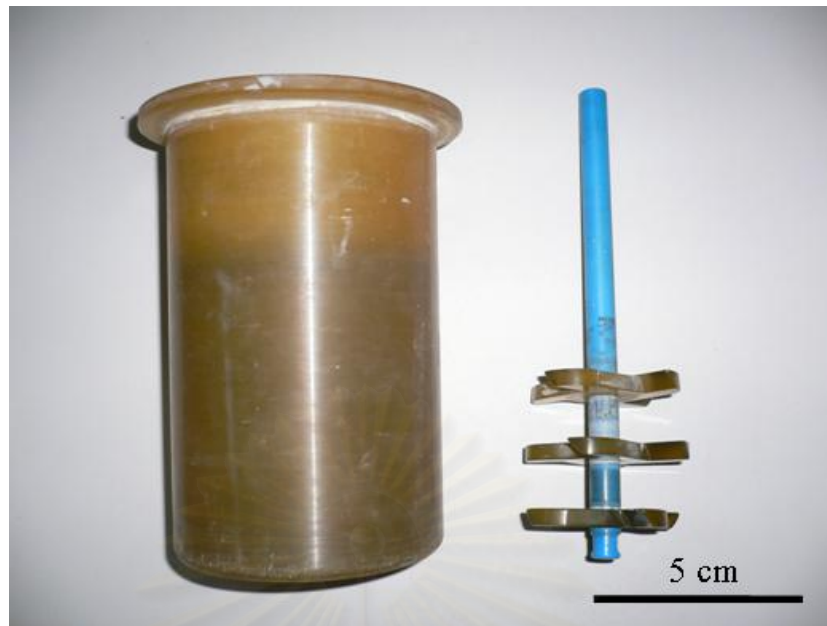
Fig. 3.5 MC nylon shaft, polyurethane blades and polyurethane container
