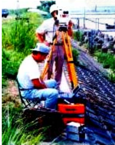
(e) Measurement of RC boat's location by total station
