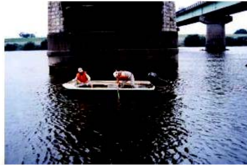
(b) Conventional investigation technique for scour from a boat
