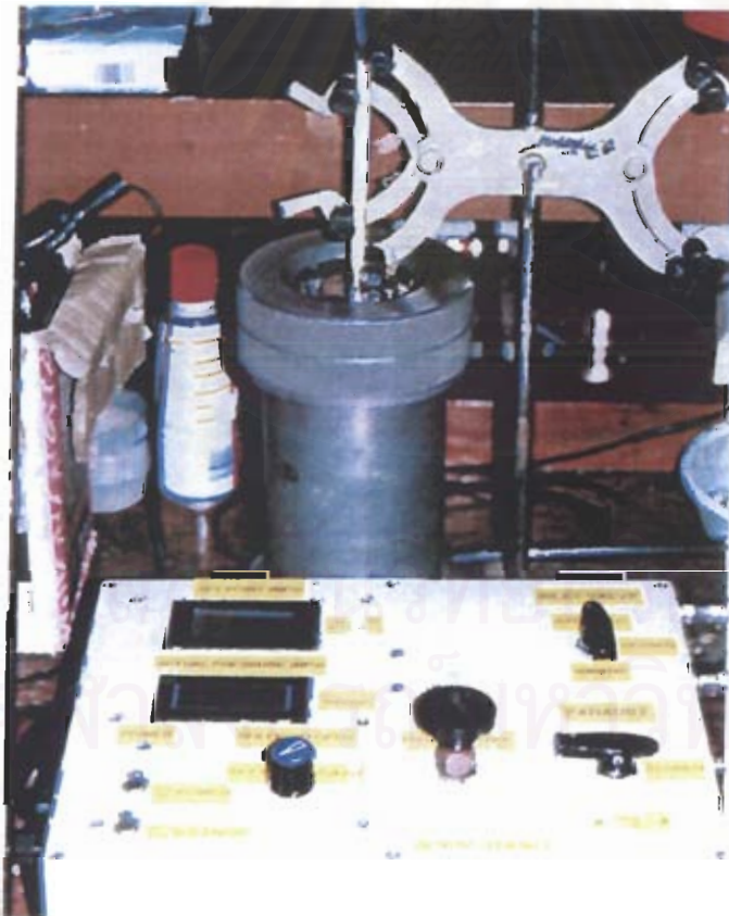
Figure 3.8 Pressure bomb technique to collect sap from shoots for generating data for pressure-volume curves.
