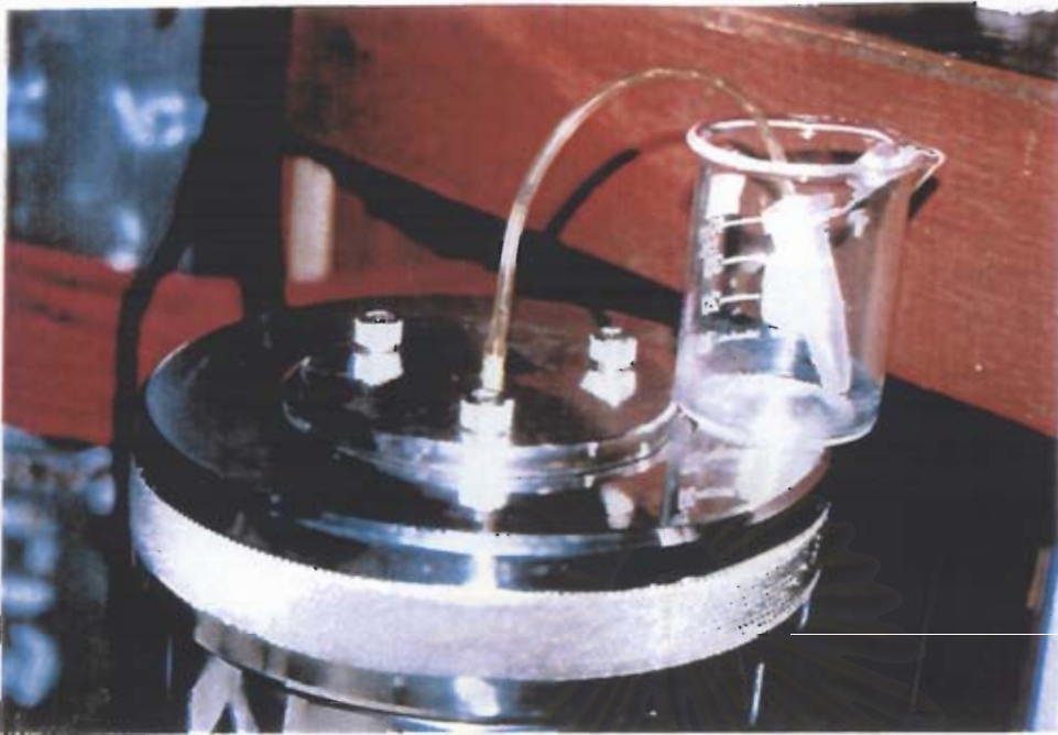
Figure 3.7 Collection of xylem sap from pressure bomb.
