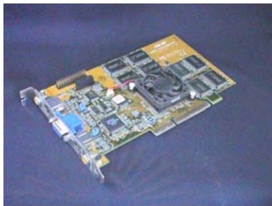
Fig. 4.1.3 Video Graphic Acceleration Card (ASUS AGP-2400TNT Model)
