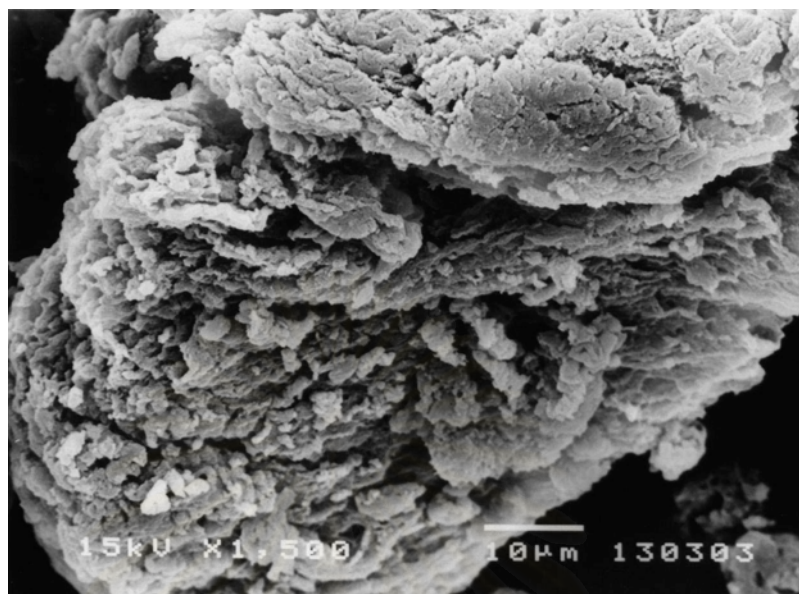
Figure 4.35 SEM photograph of the saponified starch- g -poly(acrylamide- co -maleic acid) at DR 1.71 kGy h -1 to the TD 4.0 kGy (WA = 2,256 ± 25 g g -1 )
