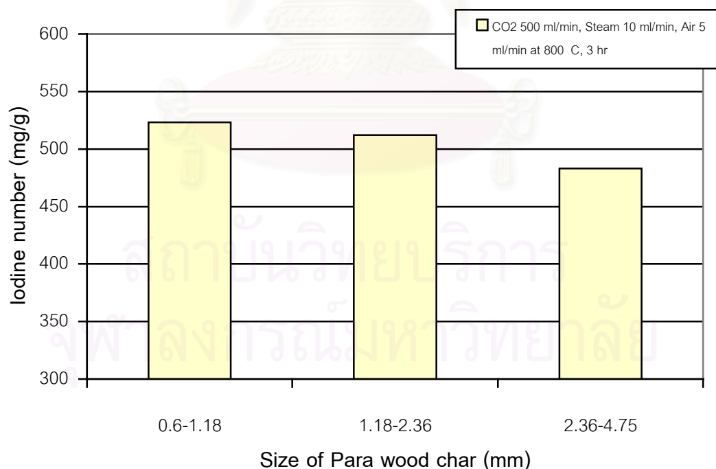
Figure 4.14 Effect of size of Para wood char on iodine number (at 800 °C, 3 hr, 9 g, CO 2 500 ml/min, steam 10 g/min and air 5 ml/min).
