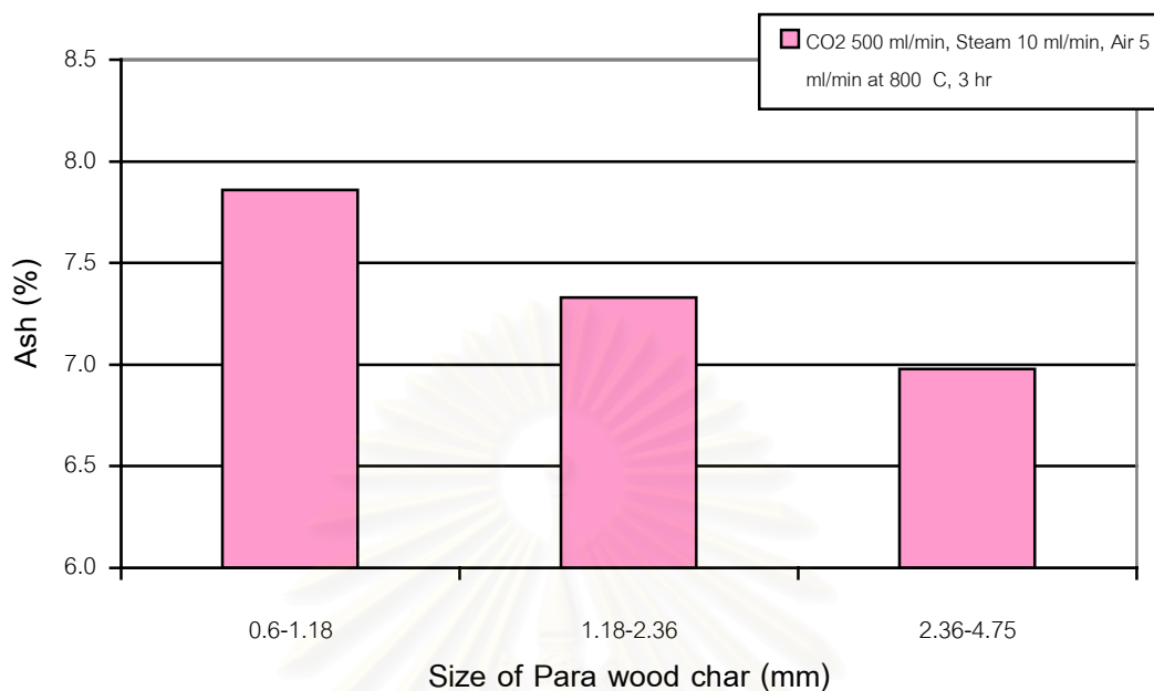
Figure 4.13 Effect of size of Para wood char on % ash (at 800 °C, 3 hr, 9 g, CO 2 500 ml/min, steam 10 g/min and air 5 ml/min).
