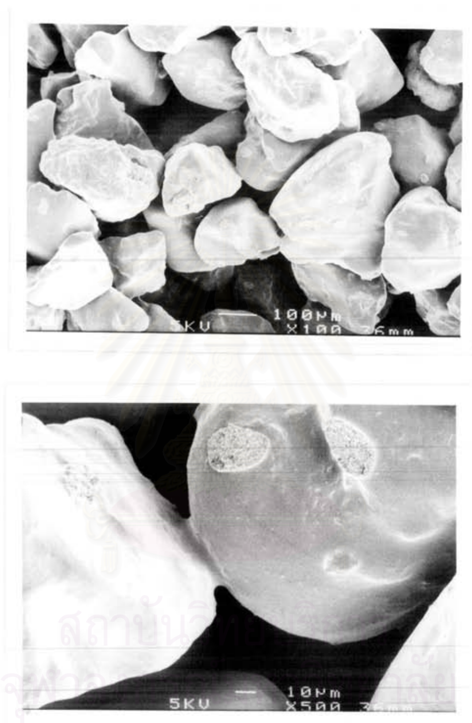
Figure 4.9 SEM micrographs of fractured surfaces (100x) and a bridge of sand grains (500x) of 1.7% FD-1 (Australian sand)
