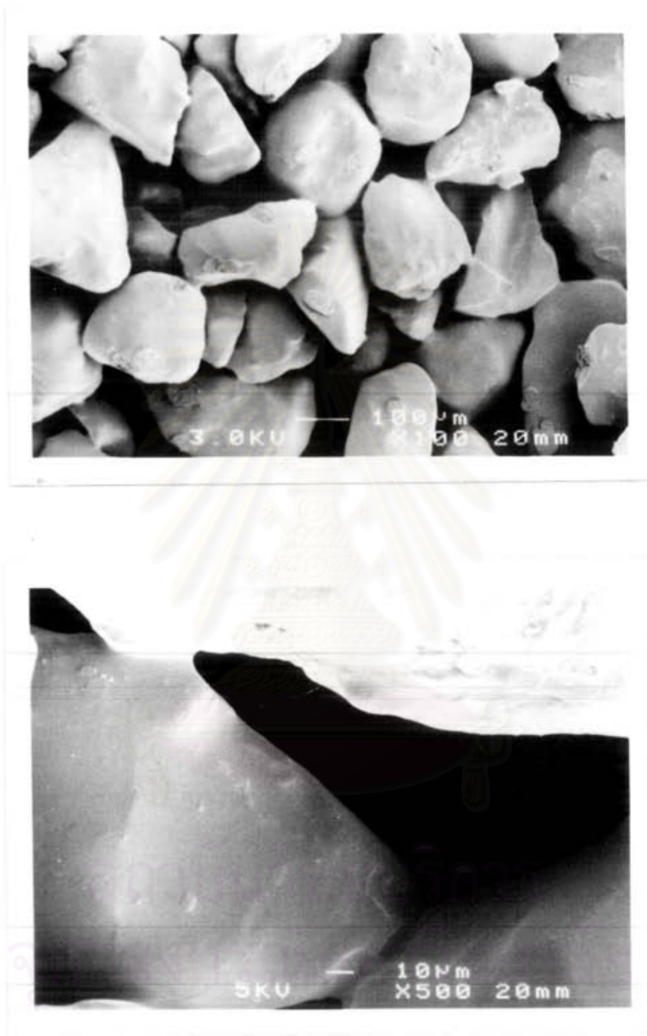
Figure 4.10 SEM micrographs of fractured surfaces (100x) and a bridge of sand grains (500x) of 2.1% FD-1 (Australian sand)
