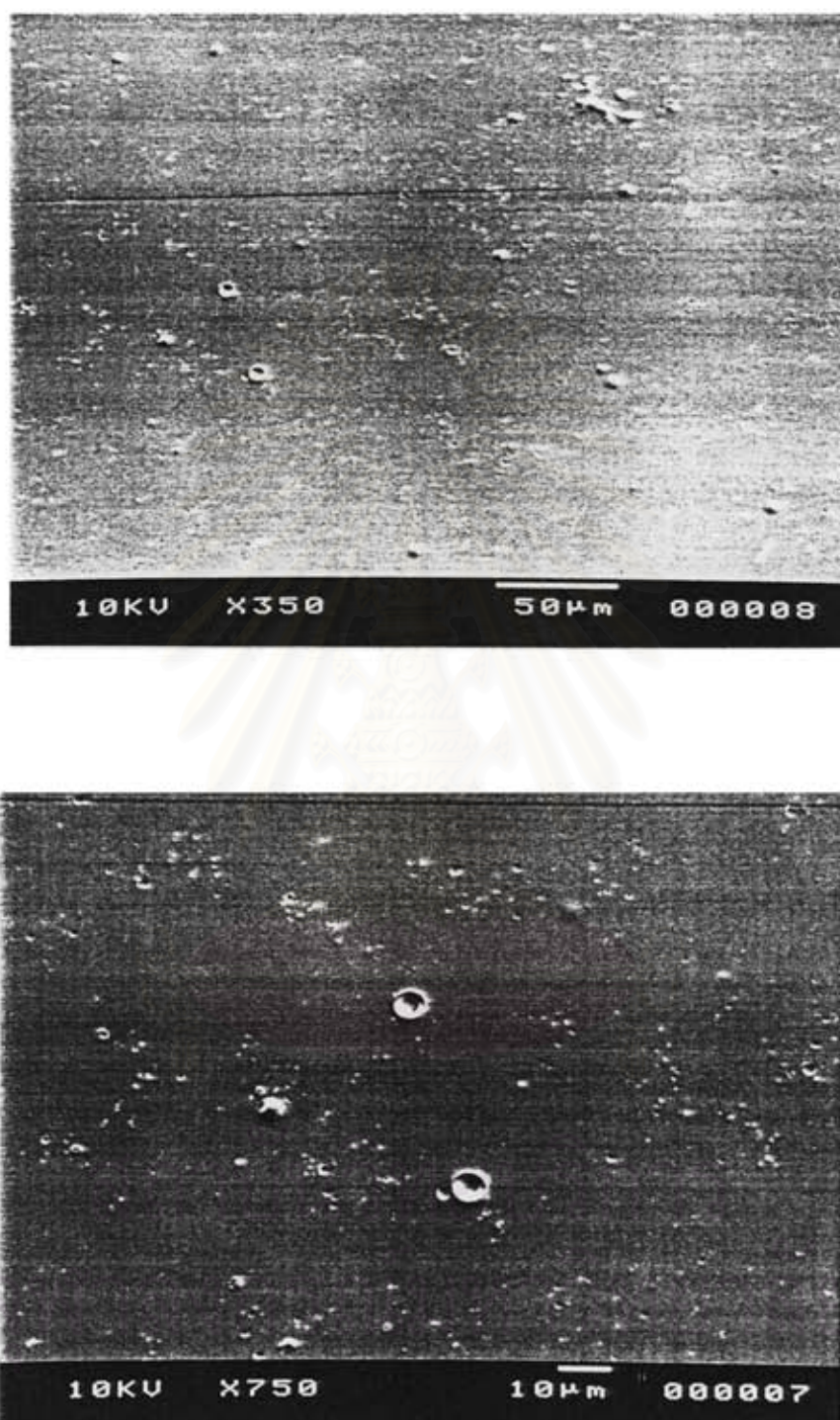
Figure 17. Surface photomicrographs of crosslinked chitosan - PVA 70,000 membrane at magnification of 350 x and 750 x (CPM 35 ; chitosan : PVA 3 : 7)
