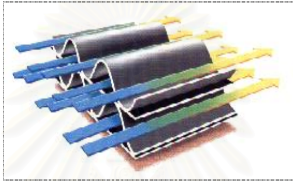
Figure 4.3 Schematic of the air stream flowing through the slots of a honeycomb rotor
