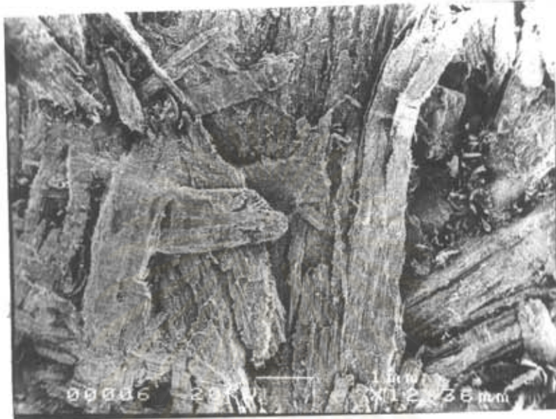
Figure 4.15 SEM micrograph of fracture surface of particleboard prepared from the flakes containing 12% moisture content with pMDI content of 7/5 (12X).
