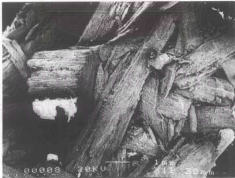
Figure 4.14 SEM micrograph of fracture surface of particleboard prepared from the flakes containing 7% moisture content with pMDI content of 7/3 (12X).
