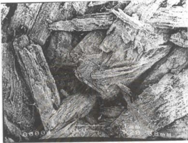
Figure 4.13 SEM micrograph of fracture surface of particleboard prepared from the flakes containing 2% moisture content with pMDI content of 7/5 (20X).
