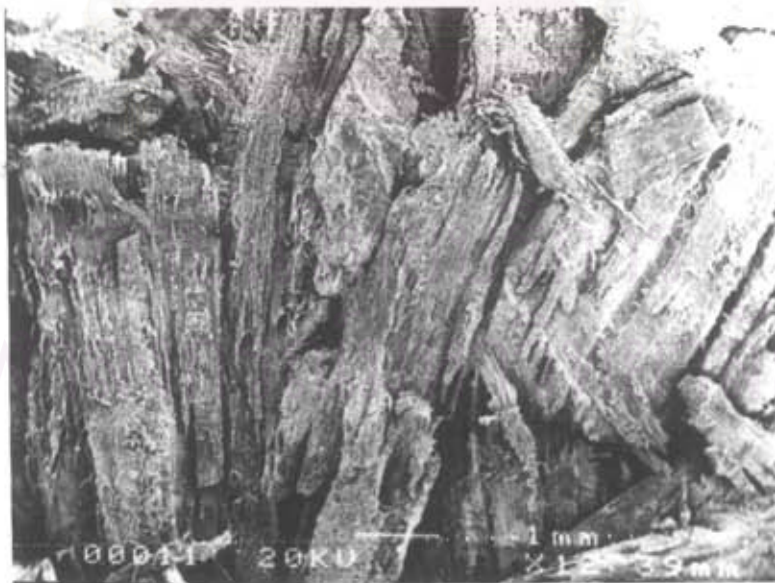
Figure 4.16 SEM micrograph of fracture surface of particleboard prepared from the flakes containing 7% moisture content with PF content of 7/5 (12X).
