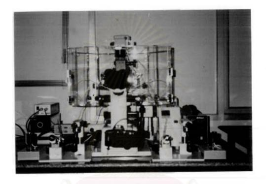
Figure 6 Arrangement of the micromanipulation set. The inverted microscope is flanked with two-side micromanipulators. Each set contains a 3D motor drive coarse control, 3D hydraulic remote fine control and a microinjector. The micromanipulator of the left is used for the holding pipette and the micromanipulator of the right is used for the biopsy pipette. The microscope is covered with a plastic incubator for environmental temperature and gas control.
