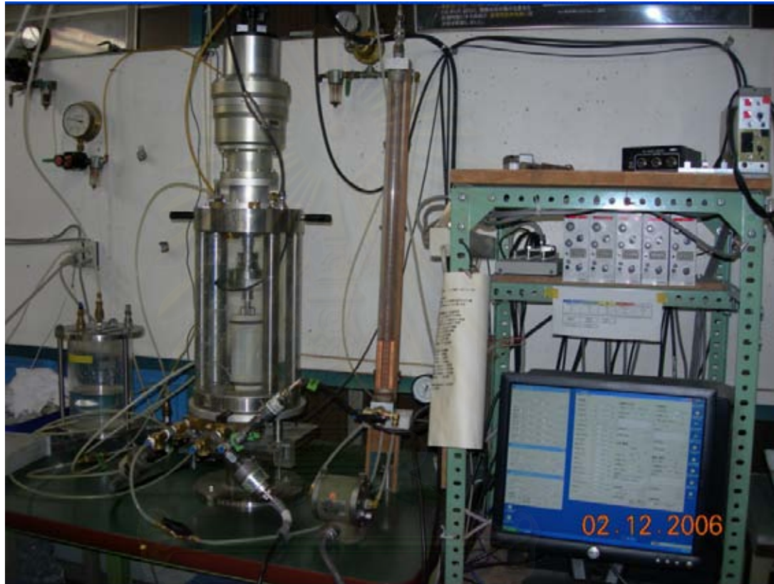
Figure B.1. Picture of Triaxial test system for carrying out the CK_0UC , CK_0DUC and CK_0UUC tests
