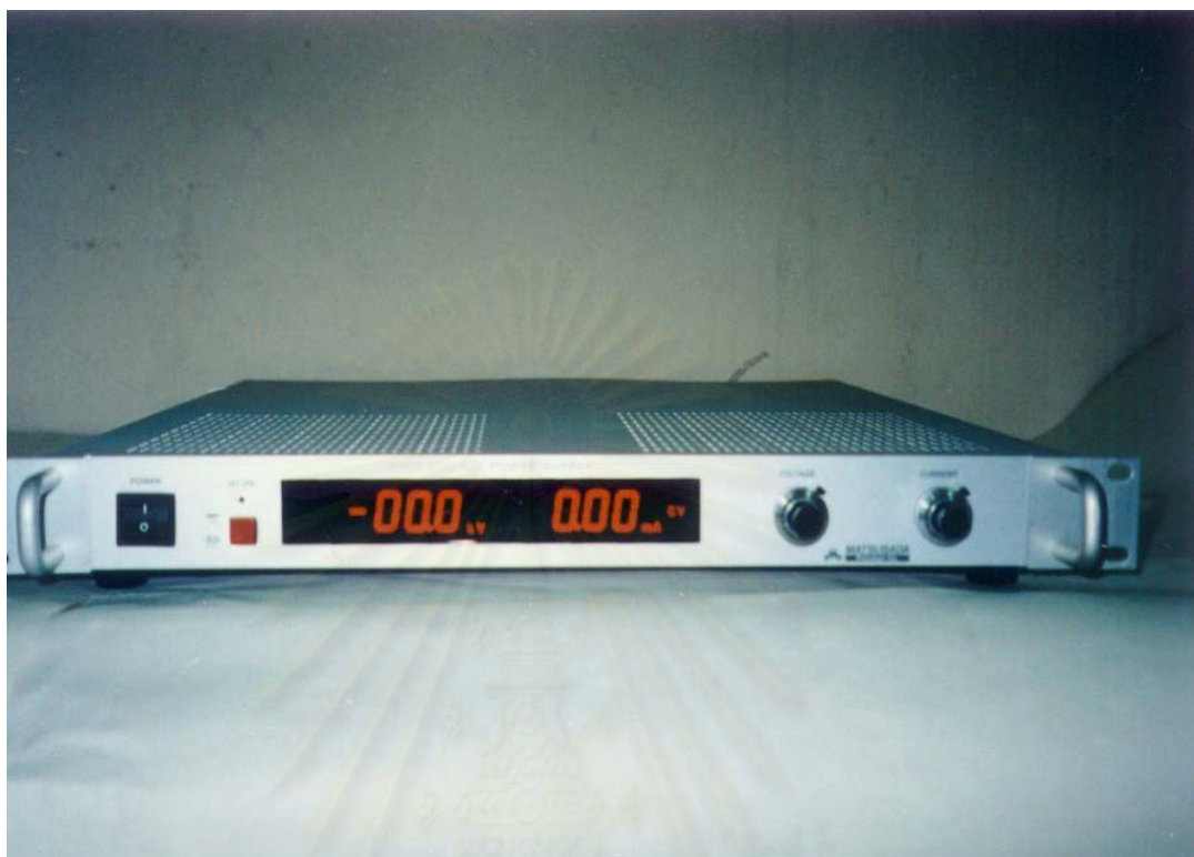
Figure 4.4 High-voltage DC generator
