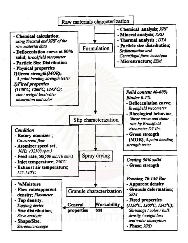
Fig.4.1 Flow chart of experiment
