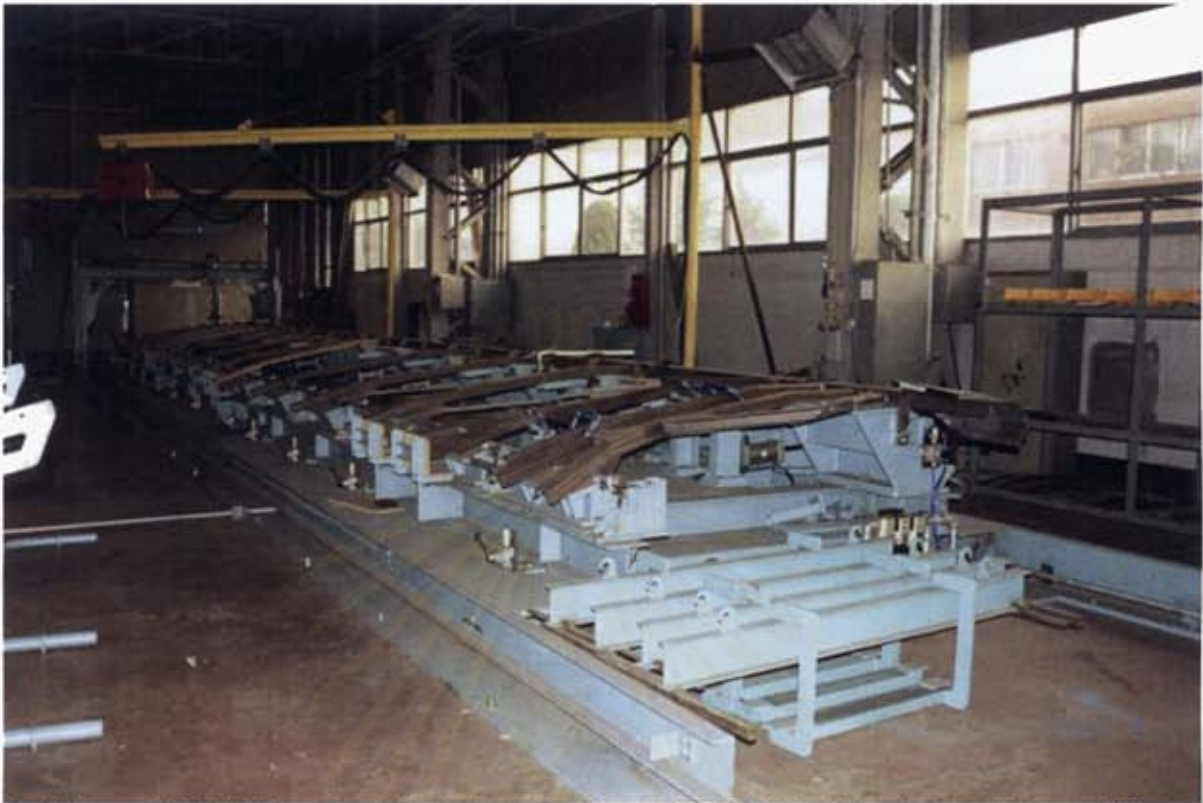
Body-side assembly jig. It is shaped to match the body curvature. The panels and their internal strengthening members are held in place by clamps while being welded.
