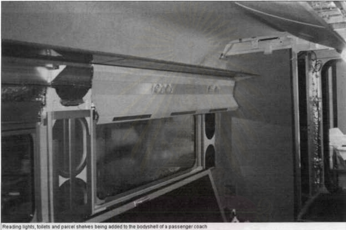
Reading lights, toilets and parcel shelves being added to the bodyshell of a passenger coach
