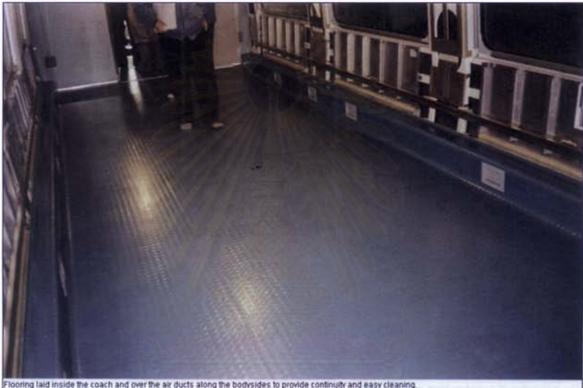
Flooring laid inside the coach and over the air ducts along the bodysides to provide continuity and easy cleaning.
