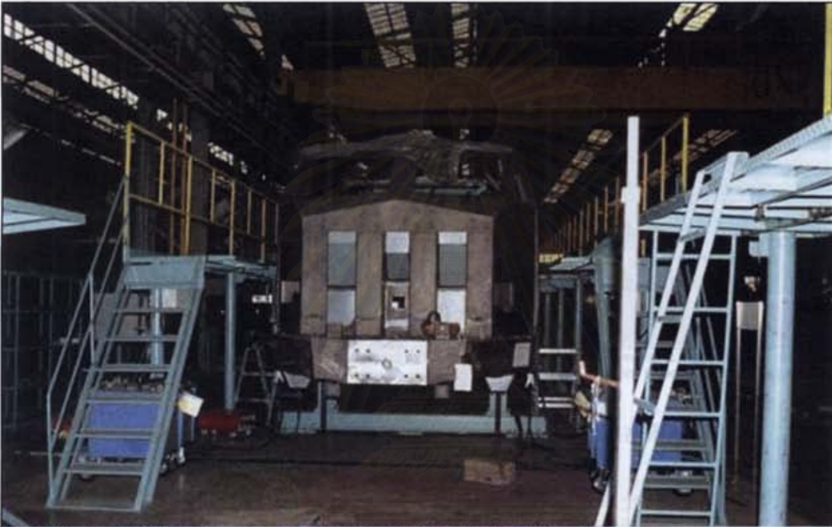
Leading end of TGV power car showing the massive steel end structure.
