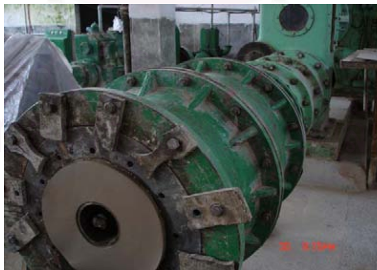
Fig. 2.21 show the extruder with central core for produced hollow product.
