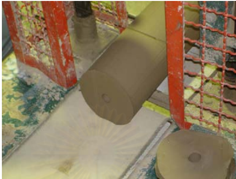
Fig. 2.20 show wire equipment for cutting clay from extrusion
