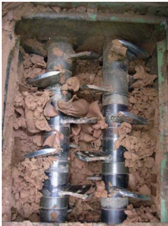
Fig. 2.18 show pug mill for mixing clay-water
