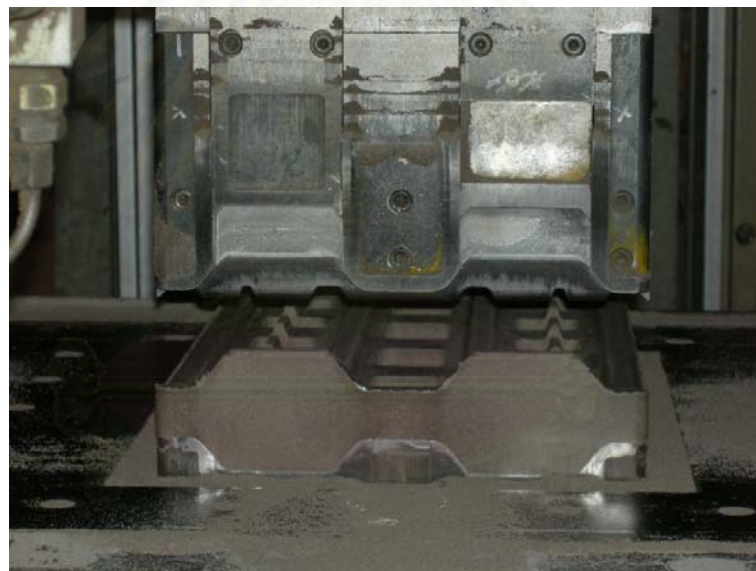
Fig 2.25 Upper and lower punch of pressing machine for cordierite kiln furniture
