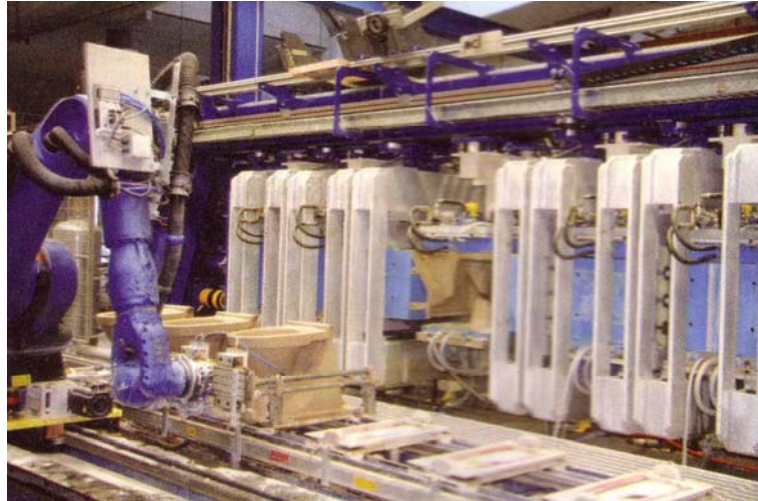
Fig 2.23 High pressure casting machine
