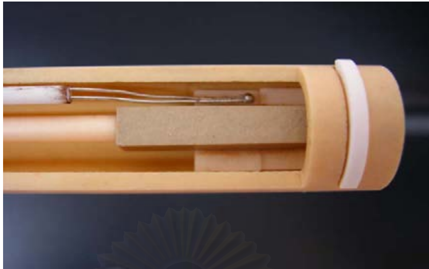
Fig 2.7 show a fused silica tube and fused silica rod of dilatometer
