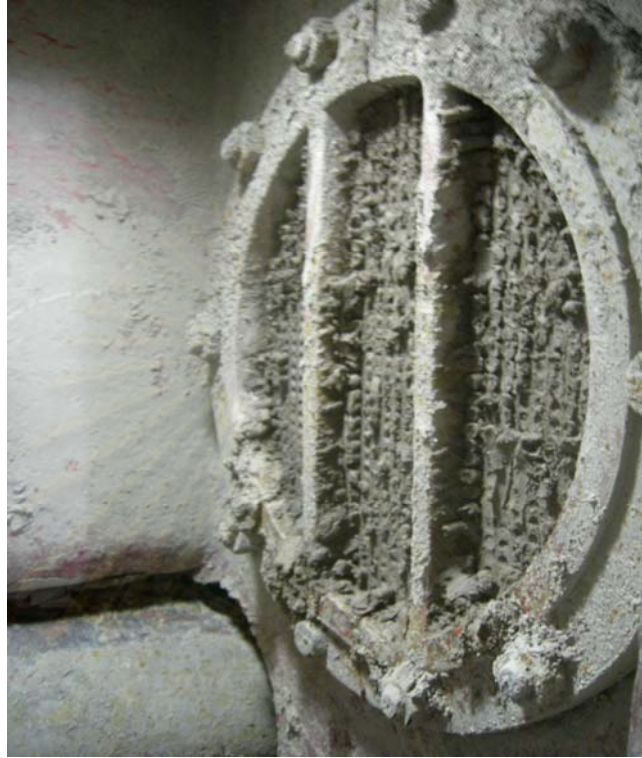
Fig. 2.19 show honey diaphragm in vacuum chamber of extruder.
