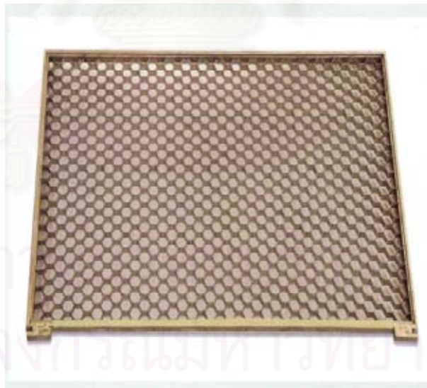
Fig 2.26 Grid inside the charger for sharing powder into the cavity mould
