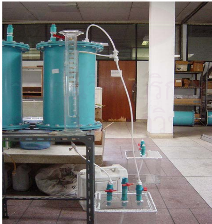
Figure 3.1 The design and operation features of the simulated landfill reactor
