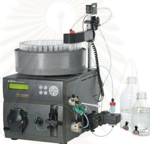
Figure 3.1 ÄKTAprime™ plus (GE Healthcare), Use for simple purification of Proteins (Figure from www1.amershambiosciences.com )
