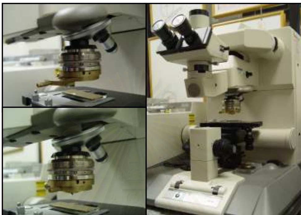
Figure 3.2 The homemade slide-on Ge \mu IRE accessory mounted onto the infrared microscope.
