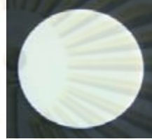
Figure 2.8 Specimen (disk) for Water Absorption, Mass Change, Diameter Change, Thickness change and Volume change
