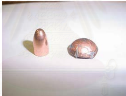
Figure 3.2: Bullet before and after impact against a 30 ply laminate (Nunes et al., 2004).
