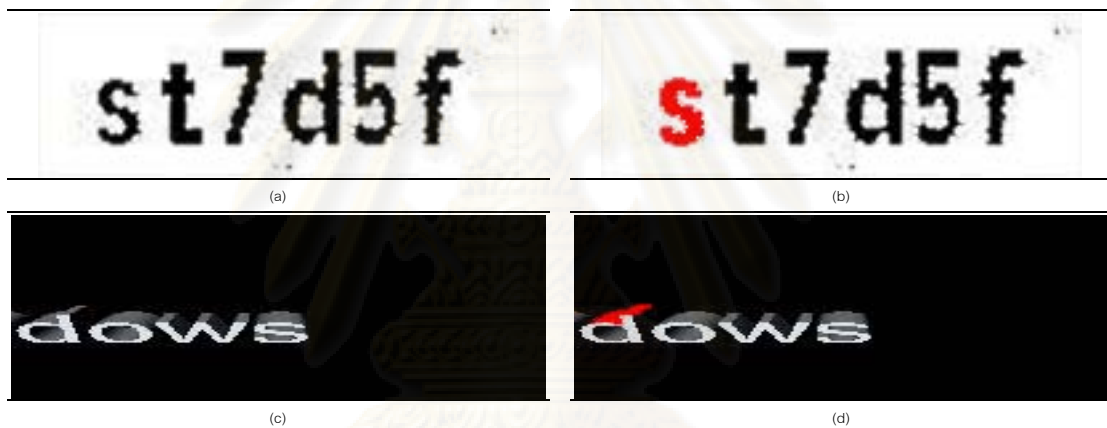
Figure 46. Examples of flood filling (a) Traditional CAPTCHA (b) Flood-filling with the first character (c) 3D animated CAPTCHA (d) Flood-filling with the proposed CAPTCHA.
