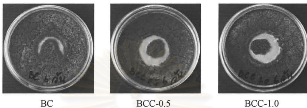
Figure 5.16 The growth of Aspergillus niger on the BC and BCC specimens, at 30°C for 6 days.
