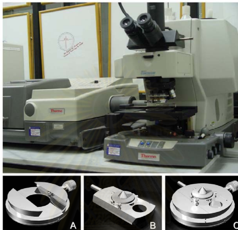
Figure B-1 The ATR FT-IR microspectrometer with homemade slide-on Ge \mu ATR accessory. (A) Ge housing, (B) the slide-on Ge \mu ATR, (C) Ge \mu ATR accessory.
