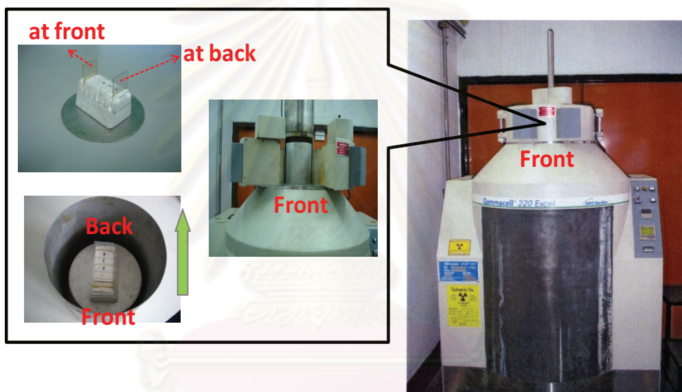
Figure 4.7: The ^{60}\text{Co} gamma radiation source (Gammacell 220 Excell).
