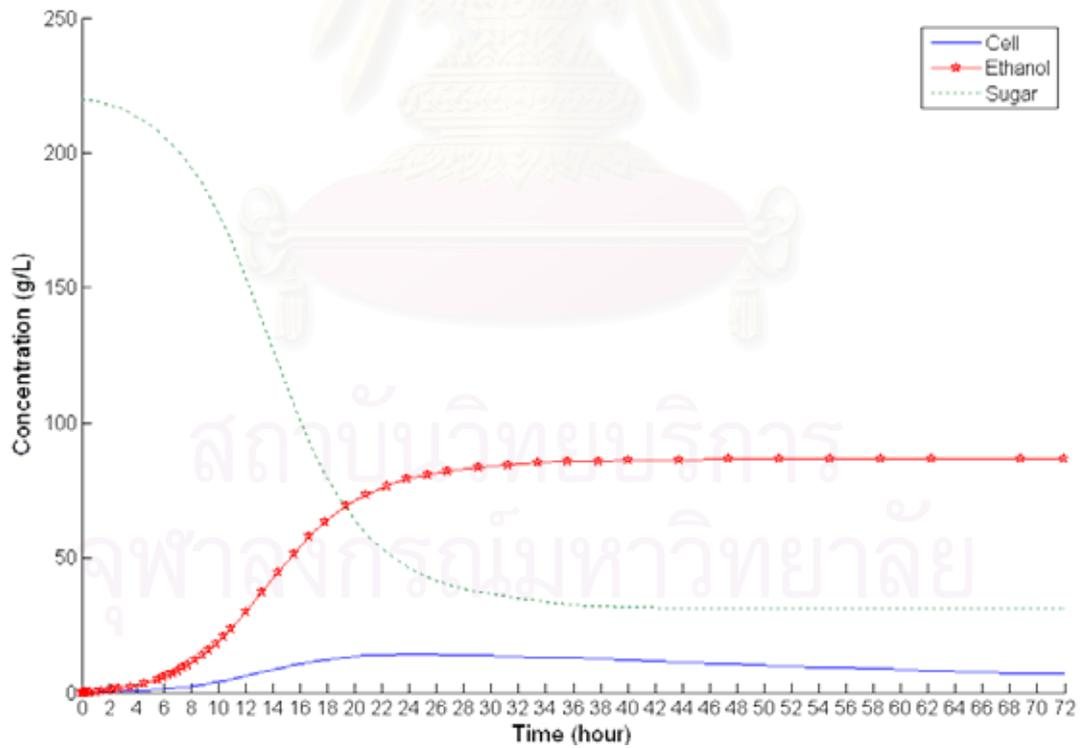
**Figure 4.9** Concentration profile in the case of decreased time interval (1 hr)
