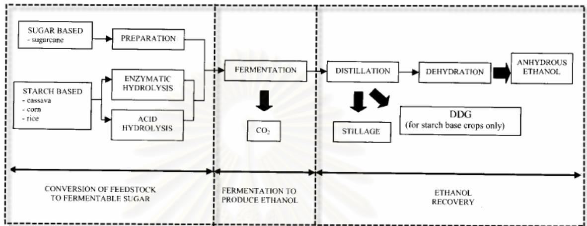
**Figure 3.1** anhydrous ethanol production processes (Yoosin et al., 2007)
