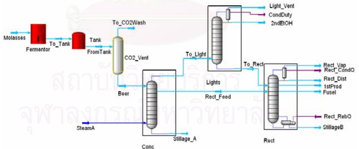
**Figure 5.1** Process flowsheet for ethanol production from molasses
