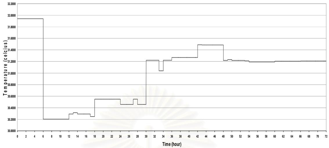
**Figure 4.8** Optimal temperature profile in the case of decreased time interval (1 hr)
