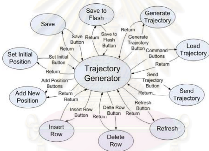
Figure 4.11: The state machine of trajectory generator menu
