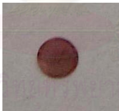
Figure 4.12 Copper grid coated with carbon films for Transmission Electron Microscopy
