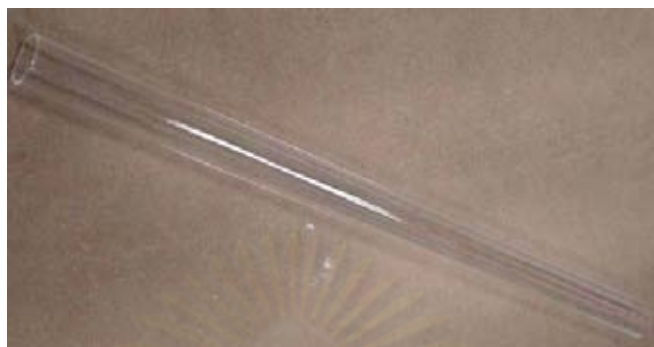
Figure 4.4 Quartz tube with inner diameter of 41 mm.
