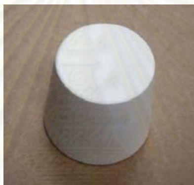
Figure 4.5 Silicone Plug for controlling leakage of gas
