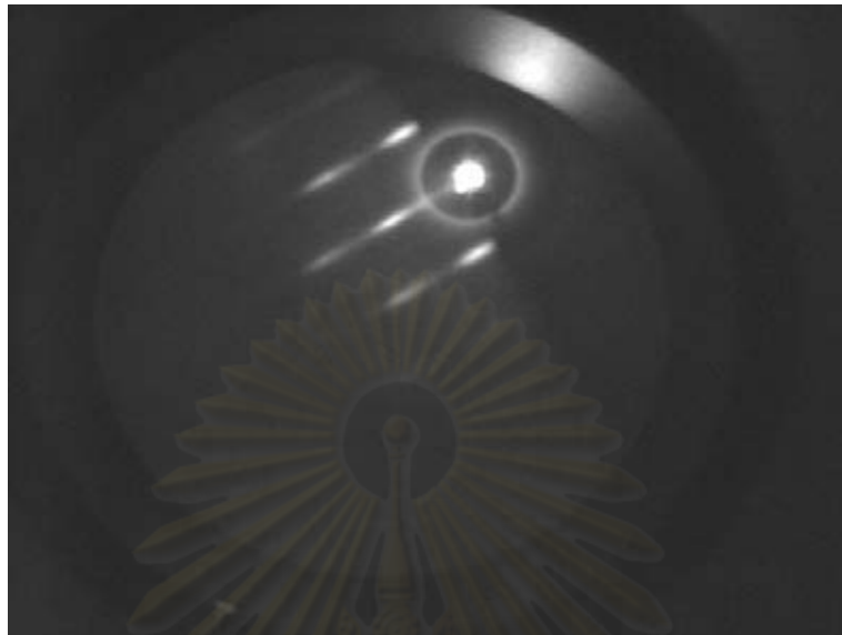
Figure 3.11 Streak RHEED pattern observed during the de-oxidation process.
