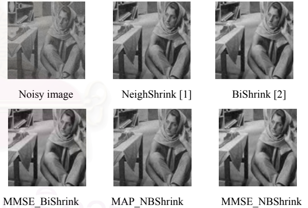
Figure 3 Image Denoising by using different methods on a Noisy image with PSNR = 18.624 (Window Size 3 \times 3 )
