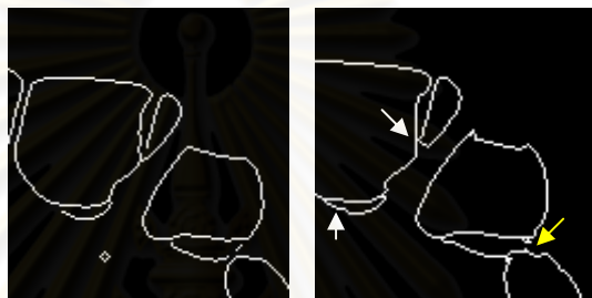
Figure 2.9: (Left) part of Canny's edge image and (Right) the interpolation in Canny's edge image by white arrow. Yellow arrow shows unexpected interpolation.
