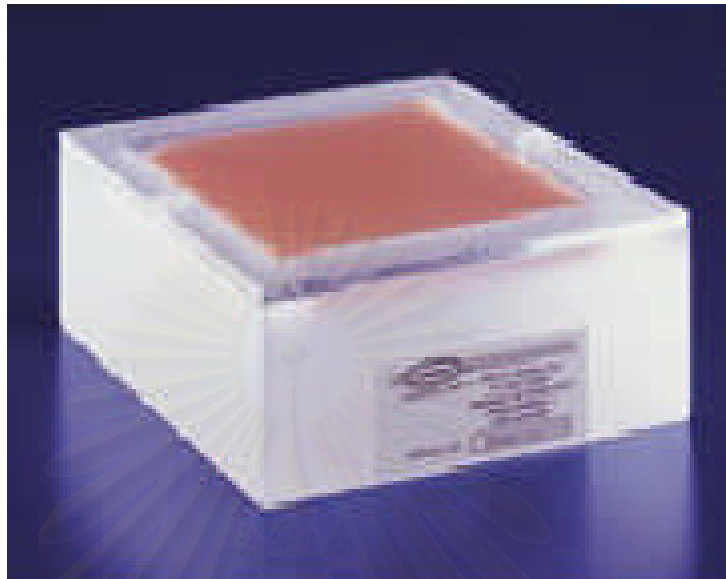
Figure 3.3 ACR Breast phantom model RMI 156
