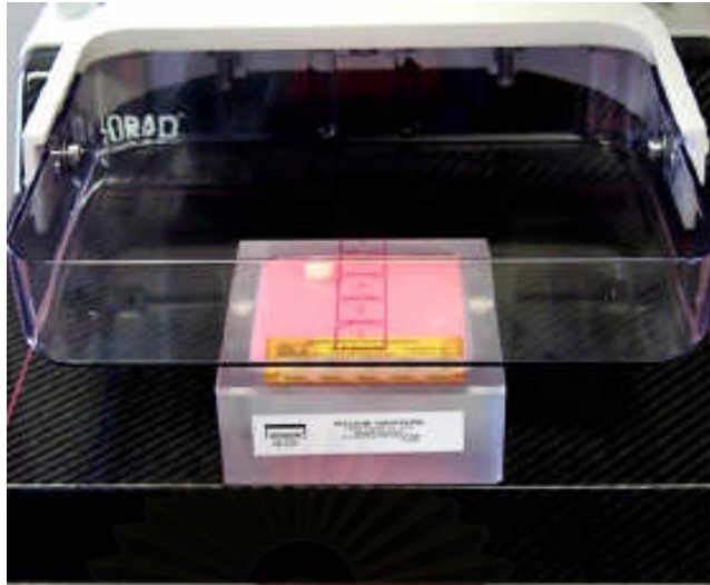
Figure 3.8 The AGD determination using ACR breast phantom
