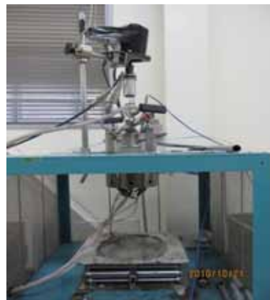
Figure 3.9 Autoclave reactor and 8 embedded heaters
