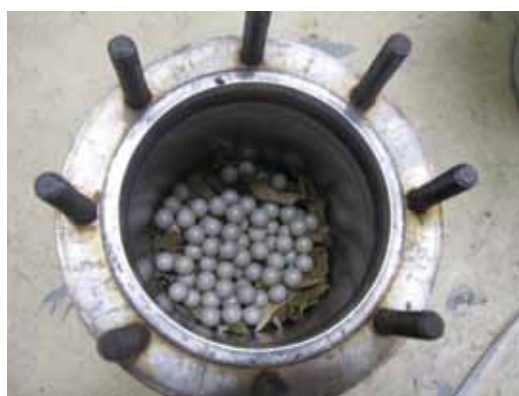
Figure 3.26 Loading raw material
