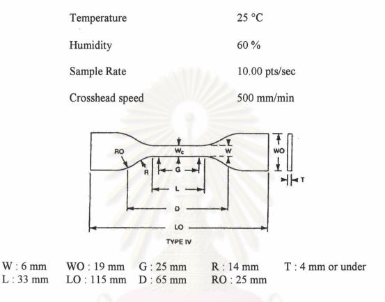
Figure 3.1 Schematic diagram of tensile test specimen (Type IV)
