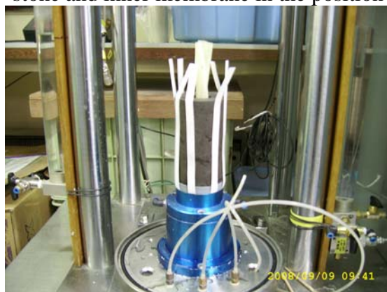
(c) Attaching 8 damp trip filter papers on the specimen wall
