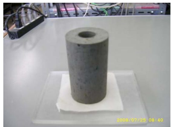
(f) A hollow cylinder specimen diameter by the wire saw ( D_i = 30 mm, D_o = 70 mm and H_i = 120 mm)
