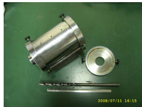
(b) Inside drilling: drill and steel mould
