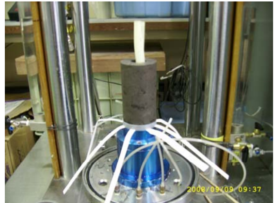
(b) Placing a specimen on the bottom porous stone
