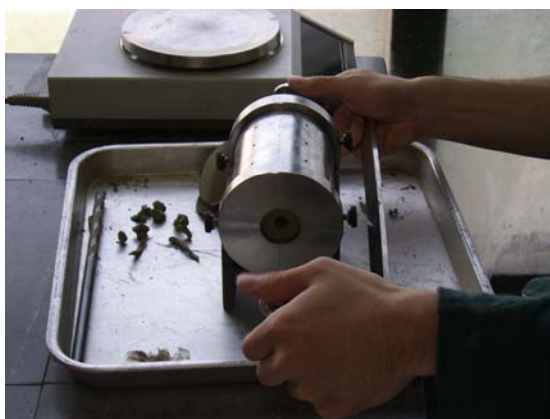
(e) Drilling inner cavity to 30 mm
