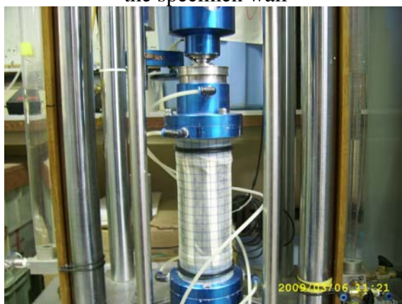
(e) Connection between load cell and top cap and potentiometer installation
