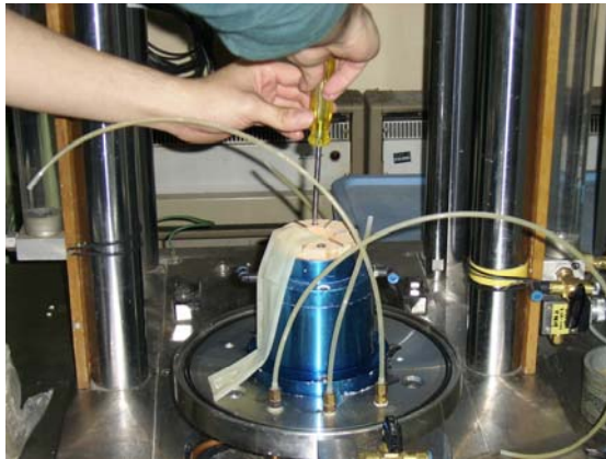
(a) Installing base pedestal, bottom porous stone and inner membrane in the position
