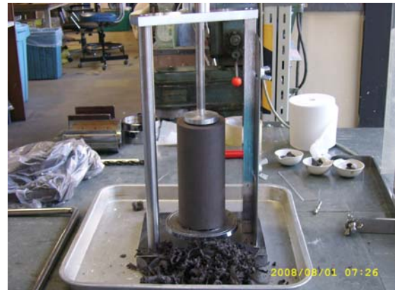
(b) Outside trimming in the soil lathe
