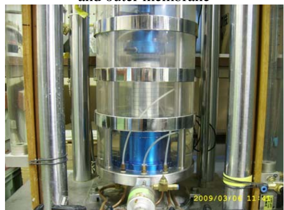
(f) Filling cell water and connection between the set of stationary and load frame
