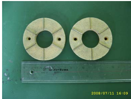
Figure 5.8 Top and bottom porous stones with radial brass blades
