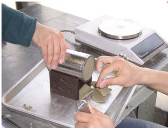
(c) Flattening the ends of sample
