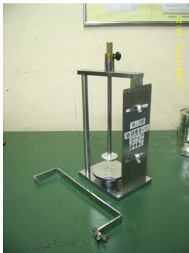
(a) Outside trimming: soil lathe and wire saw
