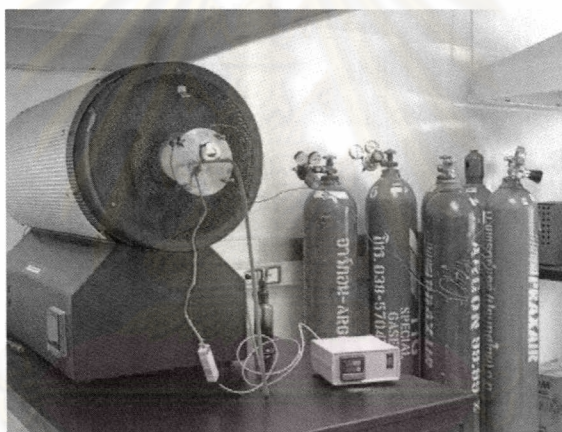
Fig. 3.2 Conventional combustion furnace and temperature measurement set up.
