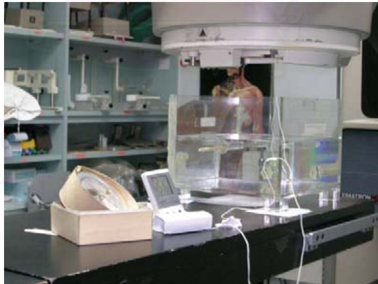
Figure 5.12 The setup of thermoluminescent dosimeter for linearity dose response 5.6.2.3 Energy response
