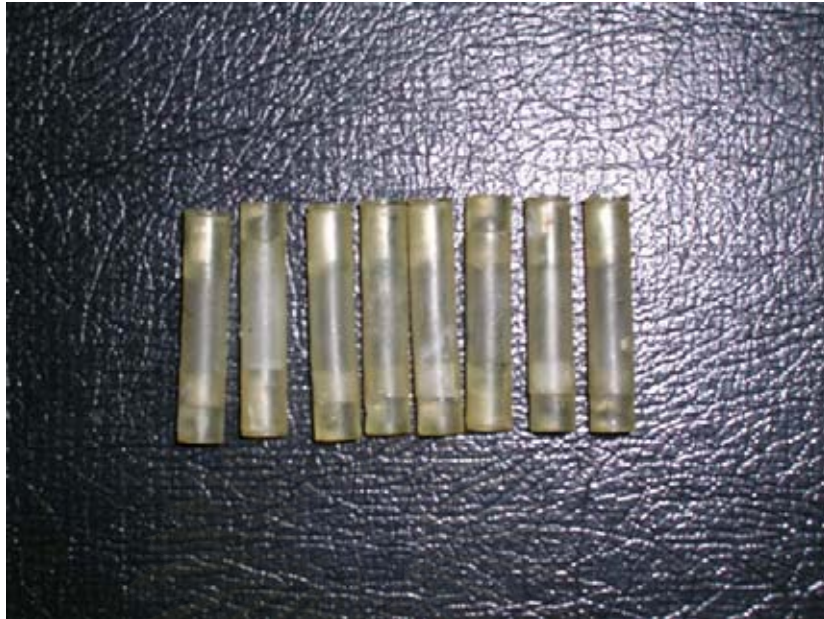
Figure 5.2 Plastic tube with thermoluminescent dosimeter chips inside
