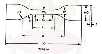
Figure 3.1 Schematic diagram of tensile test specimen (Type IV).
