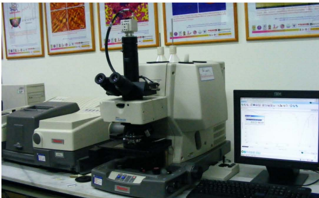
Figure 3.1 ATR FT-IR microscope: Continuum™ infrared microscope attached to the Nicolet 6700 FT-IR spectrometer.
