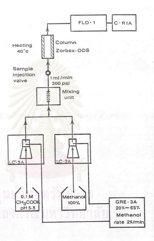
Figure 9 The flow diagram of high performance liquid chromatography (HPLC).
