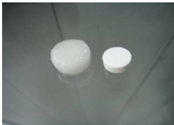
Figure 33 Image of propranolol hydrochloride matrix (F16) which prepared by using compression force 3000 PSI, after and before dissolution testing for 12 hrs. in DI water.
