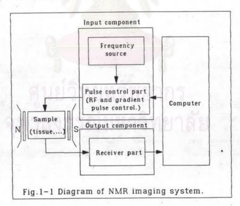
The diagram of main idea of nmr imaging is shown in Fig.1-1, the system consists of the input components - pulse control part and frequency source that take the pulsed signal to sample, the output components - receiver part that received the induced signal from the sample, and the computer which is used to control the function of the system and analyse the received signal into picture.
