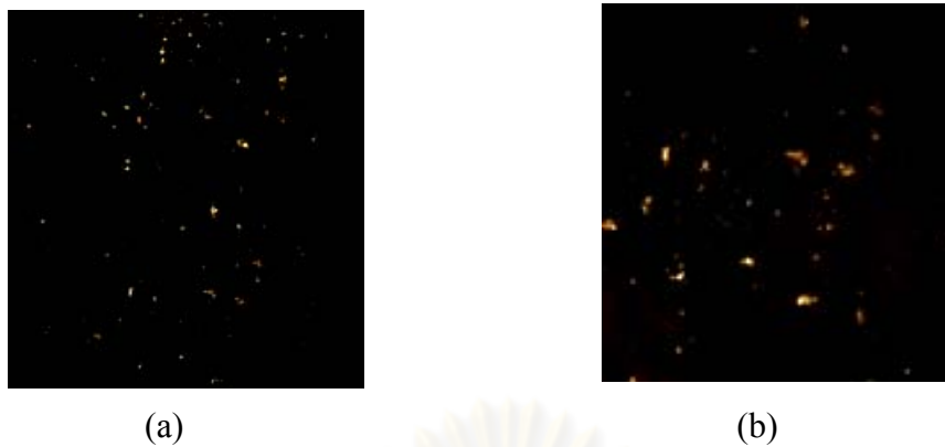
Figure 5.15 Light scattering under polarized light of liquid crystal (a) HLB 12 which contained 30 % S/C, 15 % oil and 55% aqueous phase. (b) HLB 14 which contained 36.67 %S/C, 18.33% oil and 45% aqueous phase.
