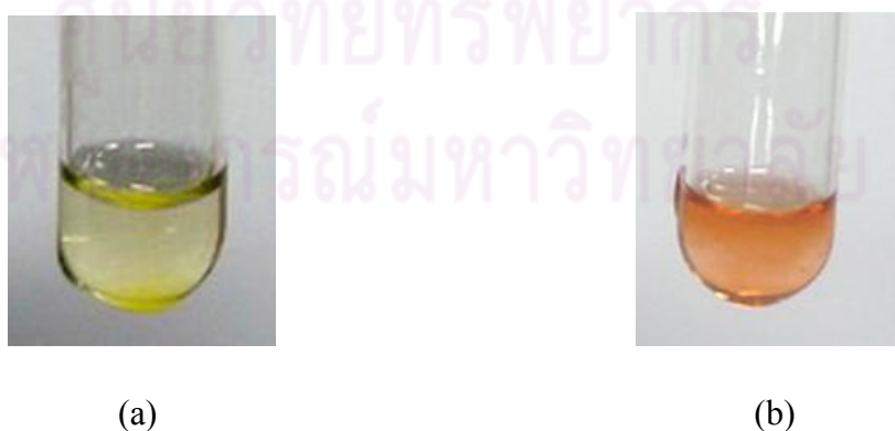
Figure 5.16 Dye solubility test (a) A w/o microemulsion after adding methyl orange, opaque solution occurred. (b) A w/o microemulsion after adding Sudan III, dye dispersed homogeneously.
