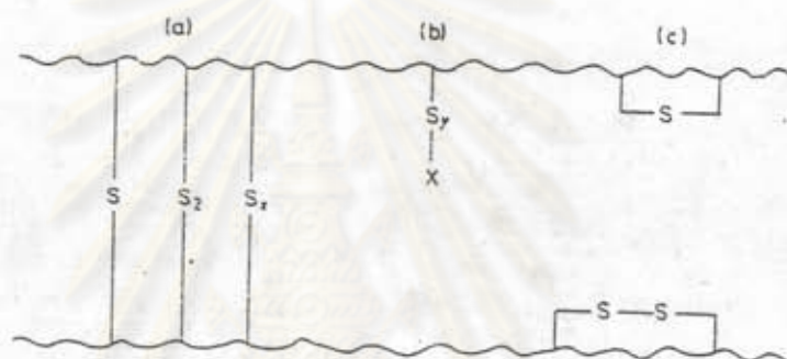
Figure 2.1 Structural features of vulcanizate network.
